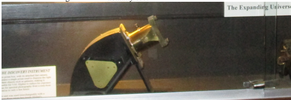
THE DISCOVERY INSTRUMENT Spectroscopy Slit Slipher's Spectroscopy Focal Plane Used To Discover The Expanding Universe. It is in the rotunda display at Lowell Observatory.
